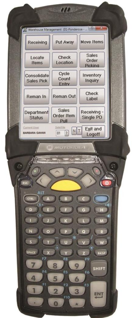
*Ponderosa utilizes durable, wireless handhelds mobile that improve the efficiency and accuracy of stocking, picking, staging, shipping, invoicing and cycle counts from the time materials arrive until they are shipped.*
